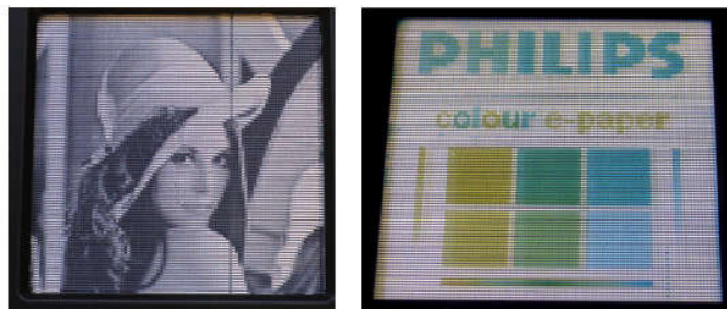
Figure 4: In-plane-switching electrophoretic display demonstrators in monochrome (left) and with a dual-particle suspension containing differently charged orange and cyan particles (right). Source: Philips Research [3].
